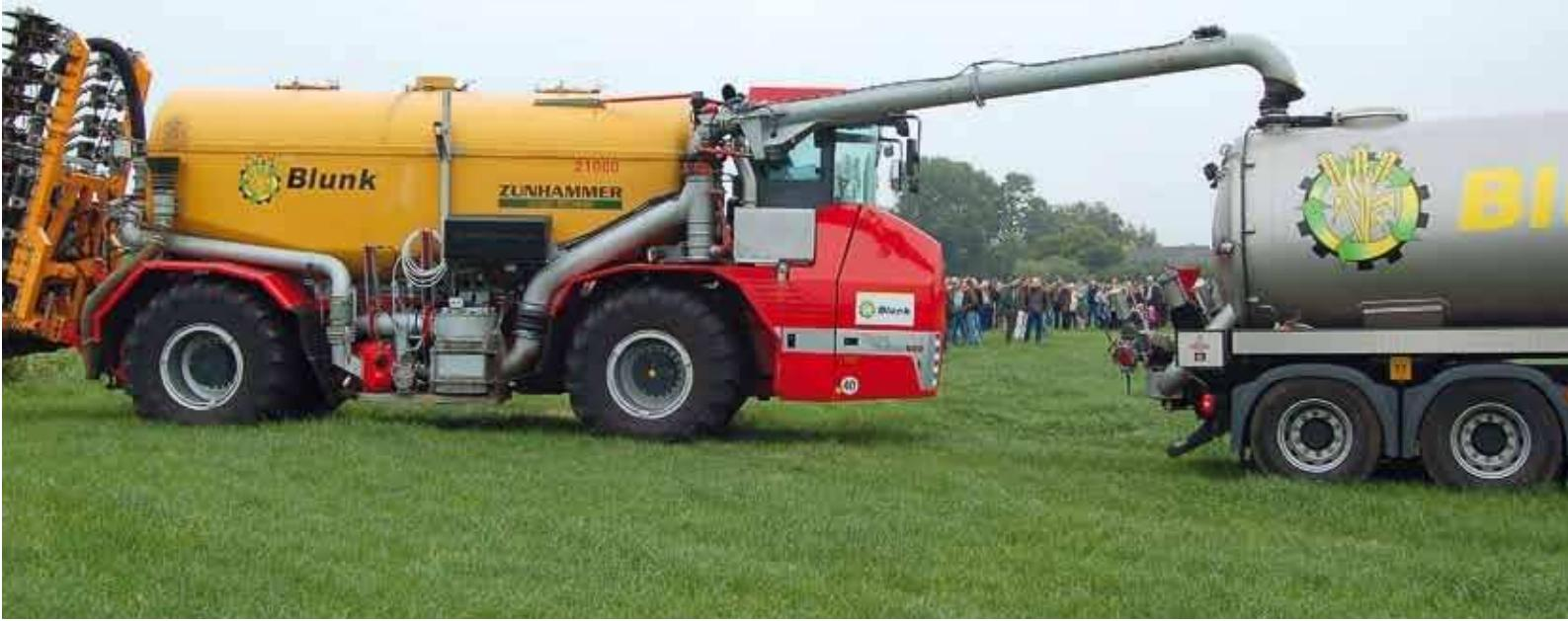
SCHLAGKRÄFTIGE GÜLLEKETTE - UMPUMPEN AM FELDGRUND VON 22 M<sup>3</sup>-VIERACHSER-LKW IN EINEN HOLMER SELBSTFAHRER.
